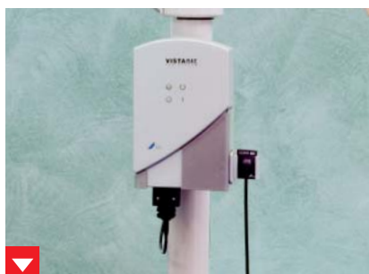
VistaRay 5 control unit in the treatment unit fitted to the lamp bar
