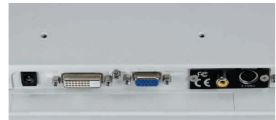
Analogue, DVI, S-Video and CVBS inputs for any video device or PC data feeds
